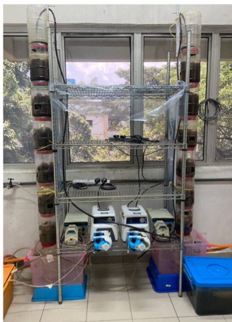
DHS reactor using polyurethane sponge as media for microorganism growth (left: clean sponge; right: biomass-enriched sponge) and its working principle.
