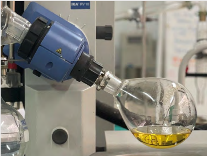
Laboratory recovery of biodiesel using rotary evaporation following transesterification of Ikan Bandaraya lipid.
