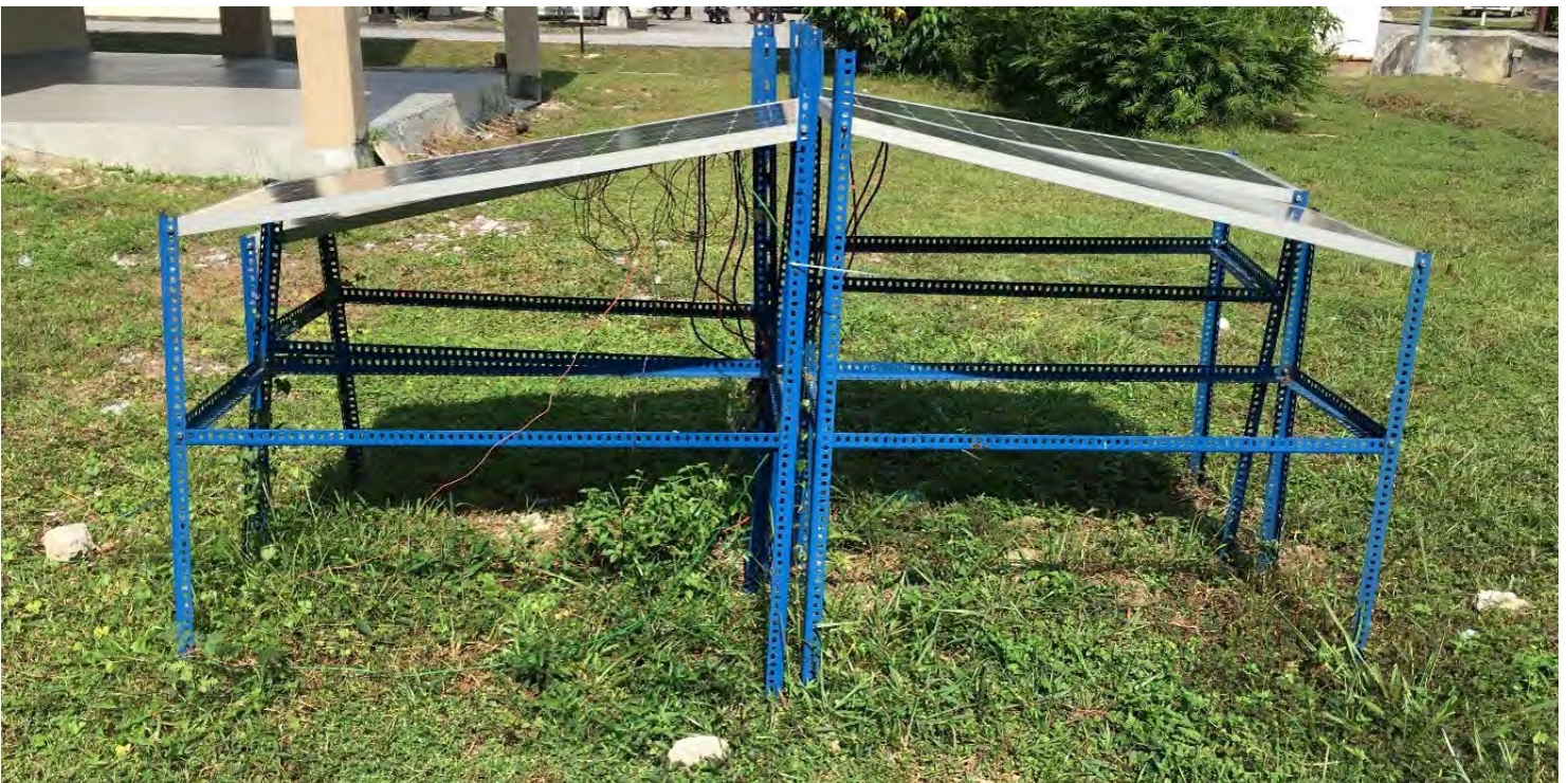
The outdoor experimental setup featuring the stationary photovoltaic frames designed to maximize tropical solar harvesting.
