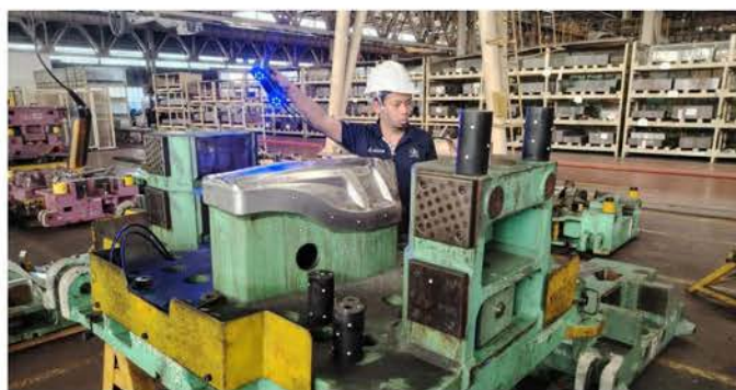
3D scanning for reverse engineering of automotive tooling conducted by ORS
