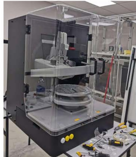
International project with Malvern Panalytical (Netherlands) to fabricate a lightweight x-ray machine by using 3D Printer
