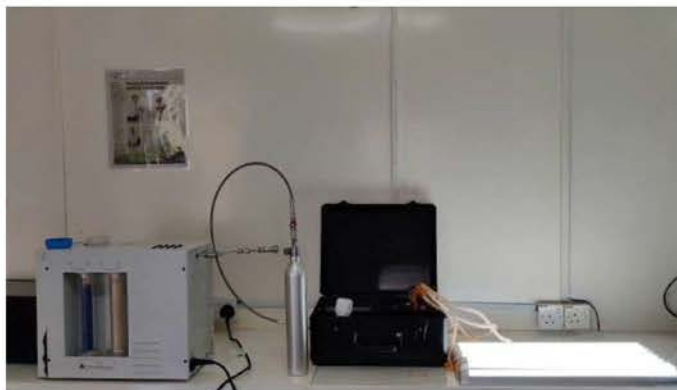
Electricity generation using a solid-state hydrogen storage system integrated with a fuel cell
